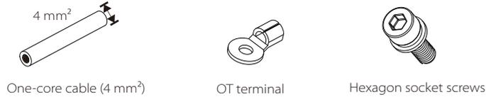
**Step 2.** Strip the grounding cable insulation (length "L2"), insert the striped cable into the ring terminal, and then clamp it.
